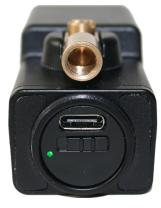
Ensure the camera is charged, the on button has been pushed to the right and that the green light is on.
