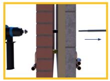
Step 3: Once through the wall, disconnect the drill bit and pull through from the inside, leaving a neat sleeve in the wall.
