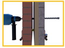
Step 2: Drill through the wall in seconds. When drilling through damp masonry, retract the drill to clear spoil.
