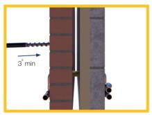
Step 1: Prepare to drill upwards at a minimum angle of 30.
